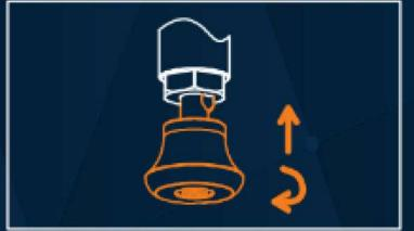
The 5 step is to rotate and lock backword the three knobs which were pulled up in the first step. Double checking they are secure and making sure the rack can not be opened.
