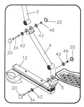
STEP 4. FIT HANDRAIL TO CONNECTING ARM (4) WITH BOLT (34), WASHER (42) & NUT (46). BE SURE TO TIGHTEN BOLT FIRMLY THEN FIT HALF MOON CAPS (20) ON BOTH ENDS.
