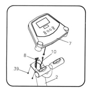
STEP 5. CONNEC<sup>†</sup>T EXTENSION CABLE WIRE (8) & GRIP PULSE WIRE (10) TO THE COMPUTER (7) THEN FIX IT ONTO HANDLEBAR POST BY USING SCREWS (39).
